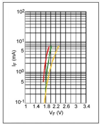
Figure 4. Typical GaAsP forward voltage vs. forward current, at +25°C.
