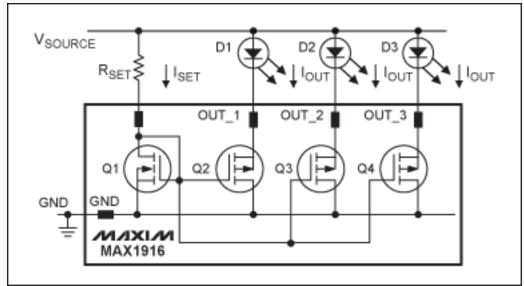
Figure 7. Simplified diagram of MAX1916 LED current mirrors.
