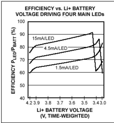
Figure 10. MAX1576 efficiency at typical lithium-battery voltages.
