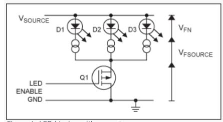
Figure 6. LED biasing with current sources.
