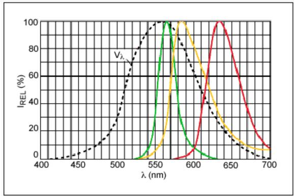
Figure 1. Relative spectral response of red, green, and yellow diodes ( $I_F = 2mA$ ,  $T_A = +25$ °C).
