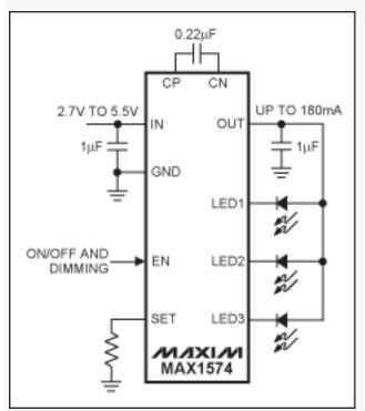
Figure 8. Integrated charge pump with one group of LED current sources.
