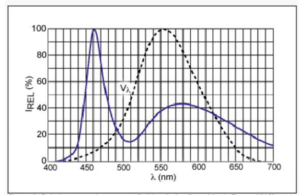
Figure 2. Relative spectral response of white diodes ( $I_F = 20$ mA,  $T_A = +25$ °C).
