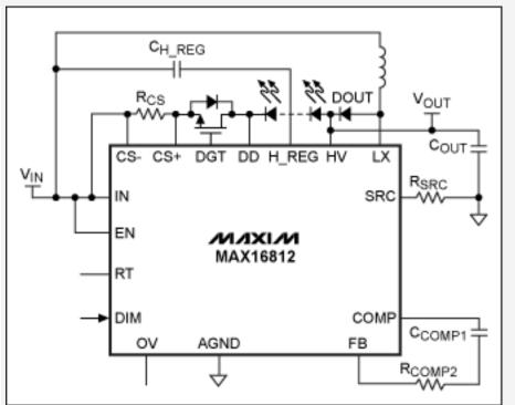
Figure 3. A buck-boost driver topology should be used in applications in which the input voltage varies above or below the total HB LED string voltage.
