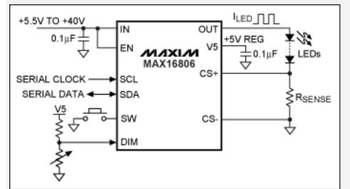
Figure 1. A 350mA linear HB LED driver IC such as the MAX16806 eliminates the need for a microcontroller or switch-mode converter.
