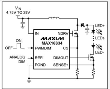
Figure 4. A boost driver with a wide, 3000:1 dimming range and built-in protection circuitry can be used for LCD backlighting in automotive infotainment applications.
