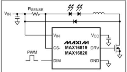
Figure 2. Using a switch-mode step-down converter driver minimizes the power dissipation and maximizes the driver efficiency in a light fixture.
