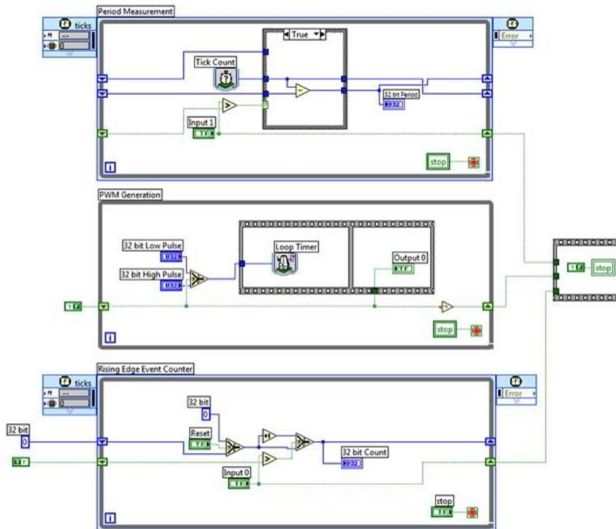
**Figure 10. LabVIEW FPGA code with parallelism becomes truly independent pathways on the FPGA silicon.**
