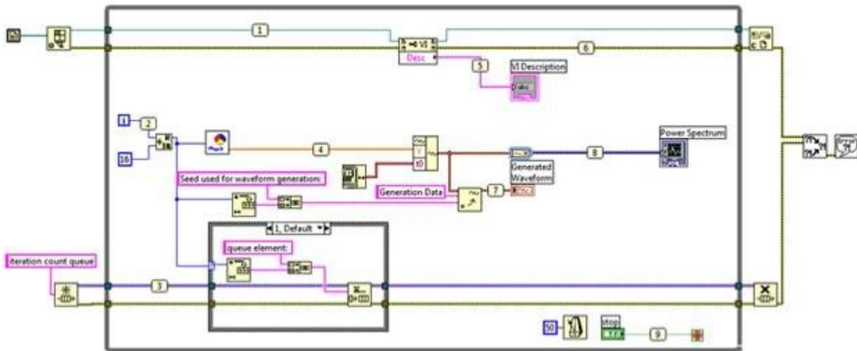
**Figure 5. Probes are effective ways in LabVIEW to see values traveling on wires throughout the application, even for parallel sections of code.**
