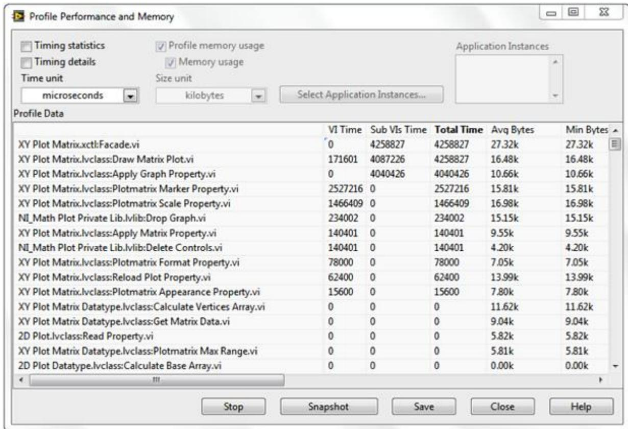
**Figure 11. Managing memory in LabVIEW is optional, but advanced users can profile memory usage to help identify portions of the application to optimize.**
