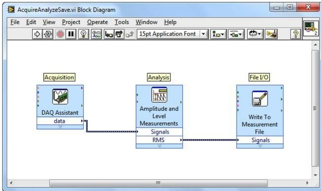
**Figure 2. Data originates in the acquisition function and then flows intuitively to the analysis and storage functions through wires.**
