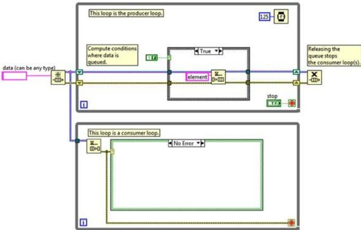
**Figure 9. The LabVIEW Producer/Consumer design pattern is often used to increase the performance of applications that require parallel tasks.**
