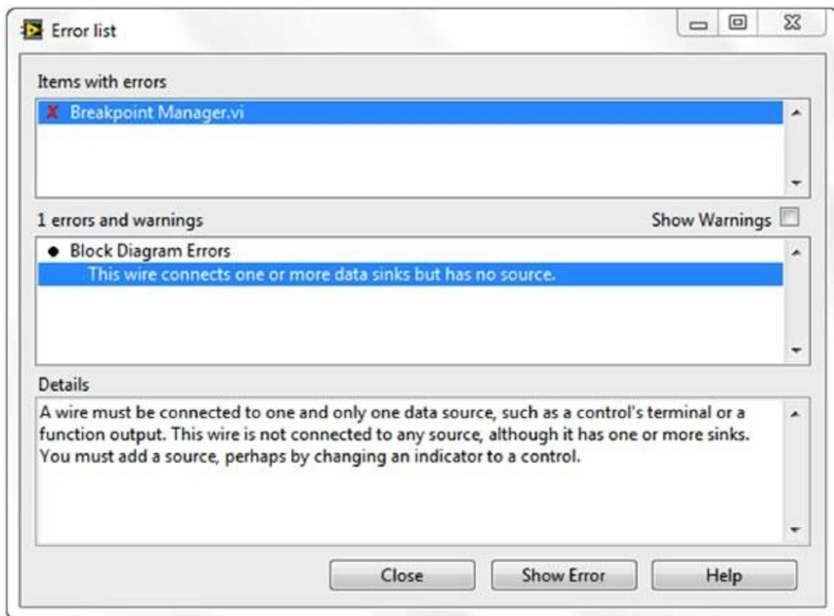
**Figure 8. The error list displays a detailed explanation of each syntax error in the entire code hierarchy.**
